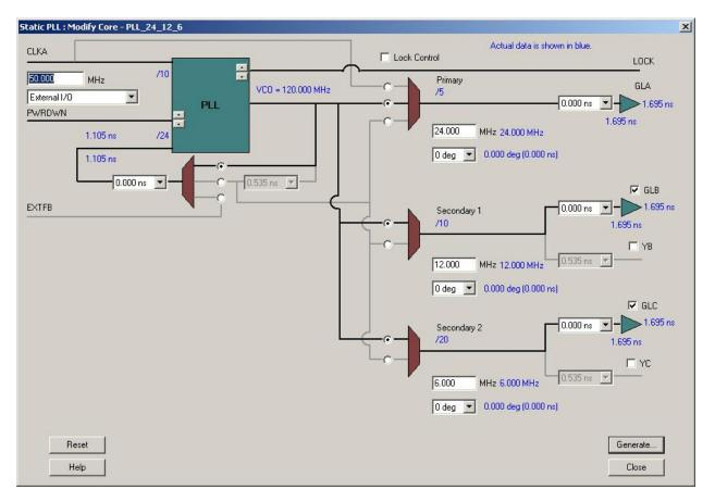
This is the static PLL wizard screen that was used for the demo. Please not that clock input is not selected as "Hardwired I/O" as the 50MHz clock is coming from Global clock pin connected to CCC without integrated PLL.
