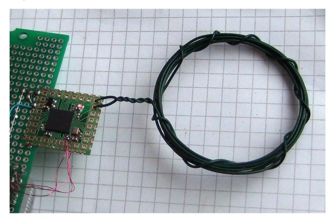
LC Oscillator test, STAMP60 rev A is used. There are no C added so only the pin capacitance is working as part of the LC circuit. For real designs some extra C should be added.
