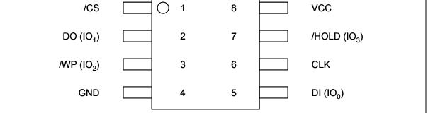
Figure 1a. W25Q64BV Pin Assignments, 8-pin SOIC 208-mil (Package Code SS)
