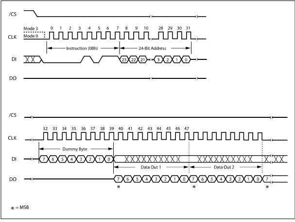
Figure 9. Fast Read Instruction Sequence Diagram
