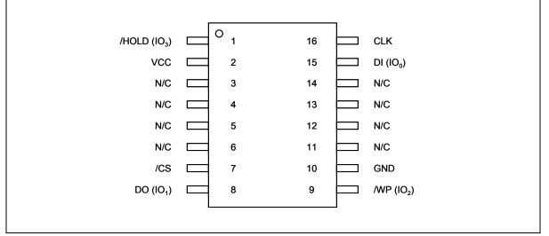
Figure 1d. W25Q64BV Pin Assignments, 16-pin SOIC 300-mil (Package Code SF)
