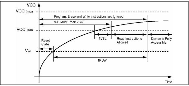
Figure 31. Power-up Timing and Voltage Levels
