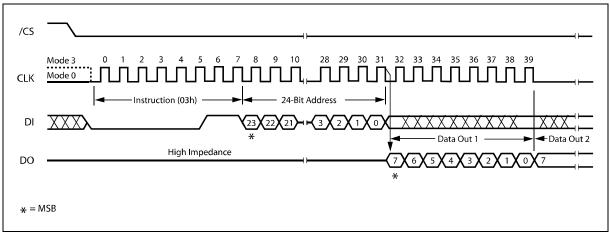
Figure 8. Read Data Instruction Sequence Diagram
