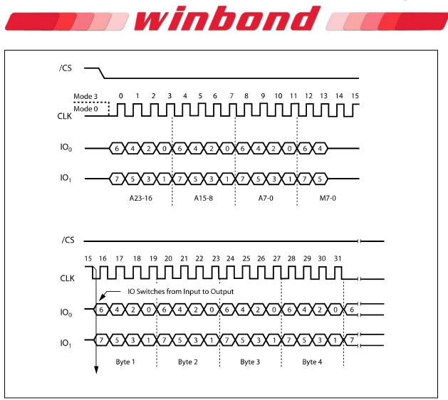
Figure 12b. Fast Read Dual Input/Output Instruction Sequence Diagram (M7-0 = Axh)
