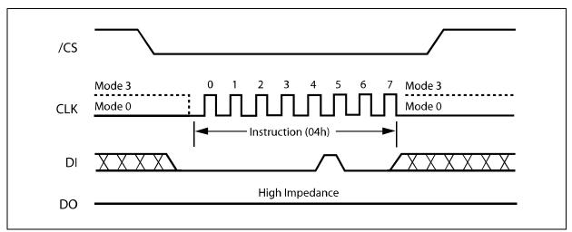
Figure 5. Write Disable Instruction Sequence Diagram
