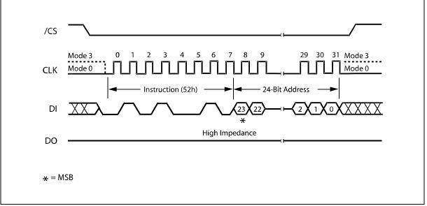
Figure 18. 32KB Block Erase Instruction Sequence Diagram
