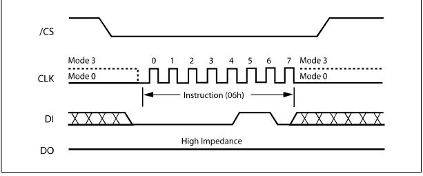
Figure 4. Write Enable Instruction Sequence Diagram
