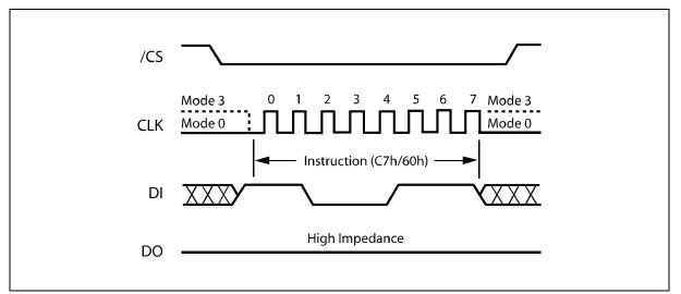
Figure 20. Chip Erase Instruction Sequence Diagram
