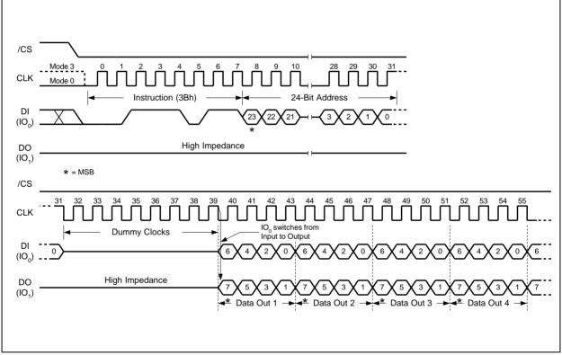
Figure 11. Fast Read Dual Output Instruction Sequence Diagram
