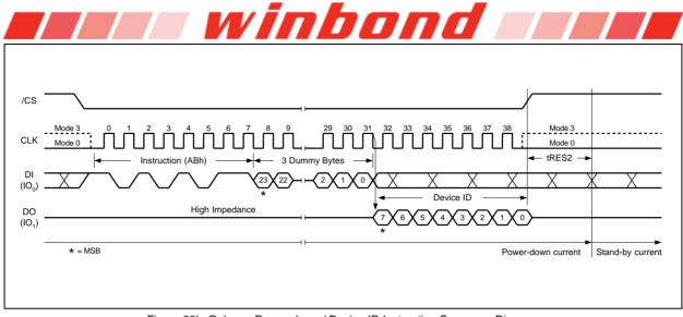
Figure 28b. Release Power-down / Device ID Instruction Sequence Diagram
