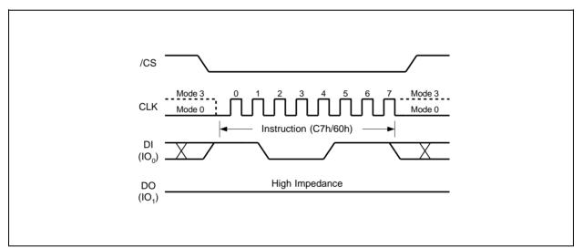
Figure 24. Chip Erase Instruction Sequence Diagram
