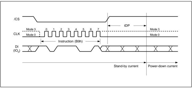
Figure 27. Deep Power-down Instruction Sequence Diagram
