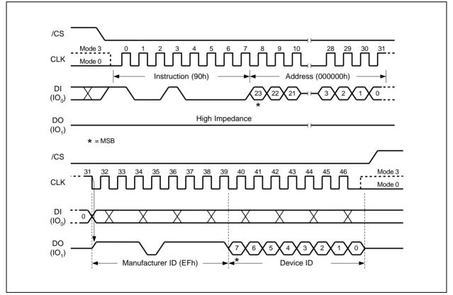
Figure 29. Read Manufacturer / Device ID Diagram
