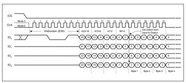
Figure 16a. Octal Word Read Quad I/O Instruction Sequence (Initial instruction or previous  $M5-4 \neq 10$ )
