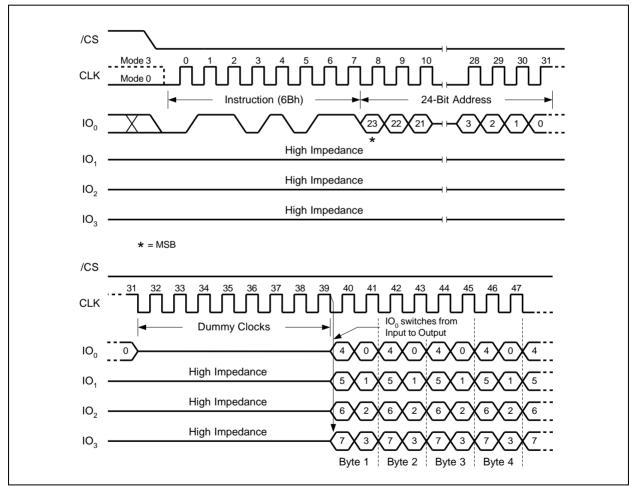
Figure 12. Fast Read Quad Output Instruction Sequence Diagram
