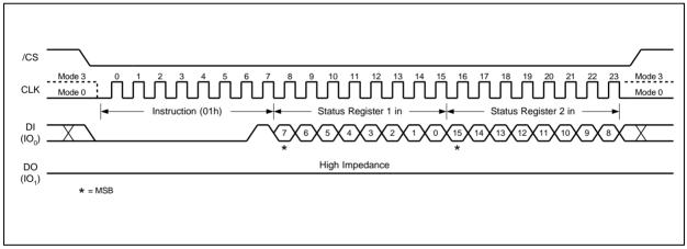
Figure 8. Write Status Register Instruction Sequence Diagram
