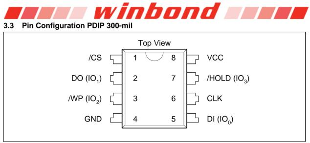
Figure 1c. W25Q32BV Pin Assignments, 8-pin PDIP 300-mil (Package Code DA)
