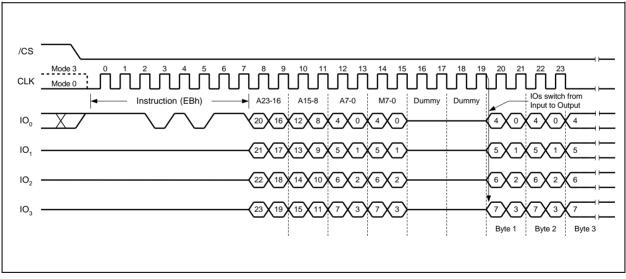
Figure 14a. Fast Read Quad I/O Instruction Sequence (Initial instruction or previous M5-4  $\neq$  10)
