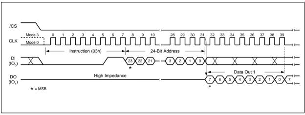
Figure 9. Read Data Instruction Sequence Diagram
