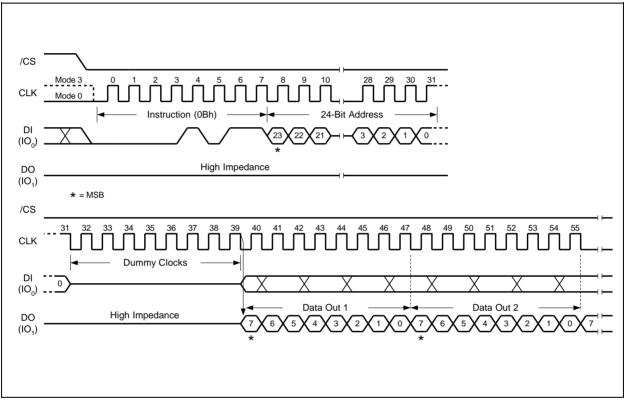
Figure 10. Fast Read Instruction Sequence Diagram
