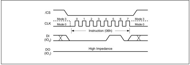
Figure 4. Write Enable Instruction Sequence Diagram
