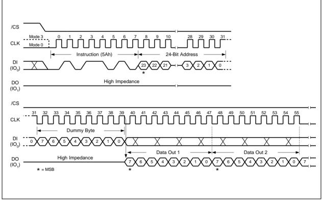
Note: 1. A23-A8 = 0; A7-A0 are used to define the starting byte address for the 256-Byte SFDP Register.
