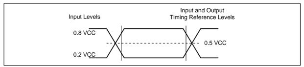
Figure 39. AC Measurement I/O Waveform
