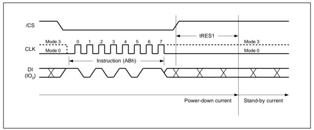
Figure 28a. Release Power-down Instruction Sequence
