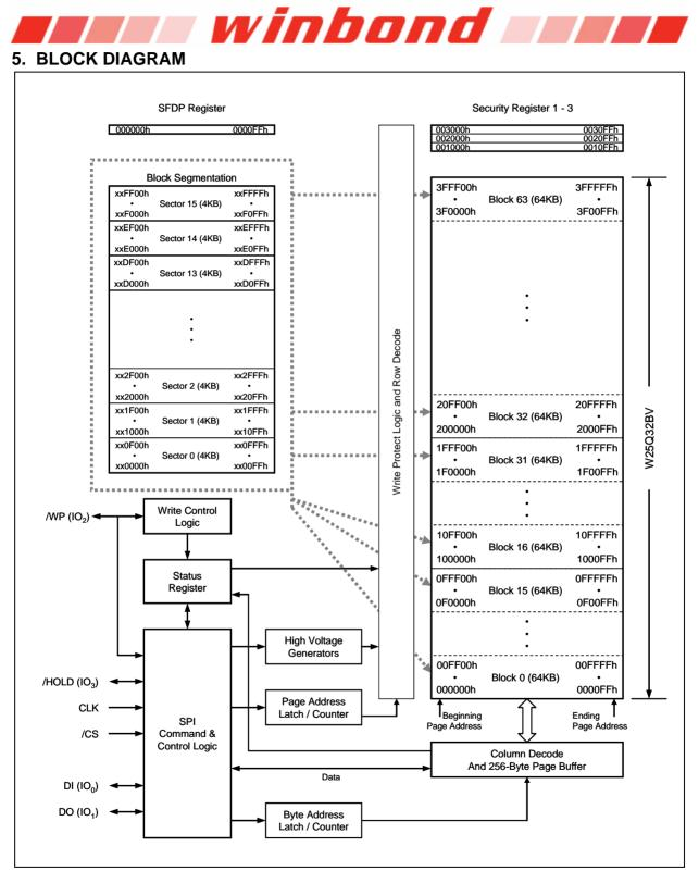
Figure 2. W25Q32BV Serial Flash Memory Block Diagram
