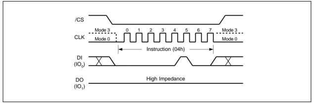
Figure 6. Write Disable Instruction Sequence Diagram
