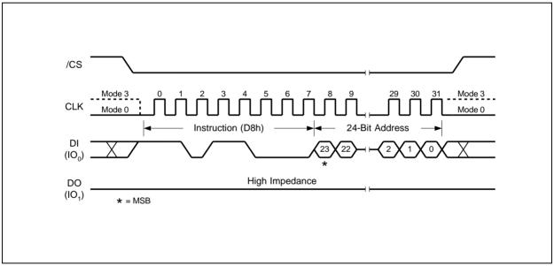
Figure 23. 64KB Block Erase Instruction Sequence Diagram
