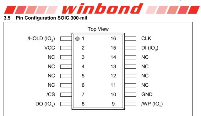
Figure 1d. W25Q32BV Pin Assignments, 16-pin SOIC 300-mil (Package Code SF)
