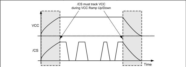
Figure 38b. Power-up, Power-Down Requirement
