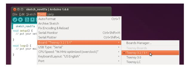
Step #4: Verify an example to make sure Arduino can compile the workshop files.
