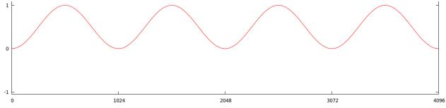
Window functions destroy about half of the original data, where they multiply by zero or very small numbers. For this reason, the Teensy Audio Library uses 50% overlap in its **fft1024** object. Twice as many 1024 point FFTs are computed, where the second set uses the window function offset by 512 points.
