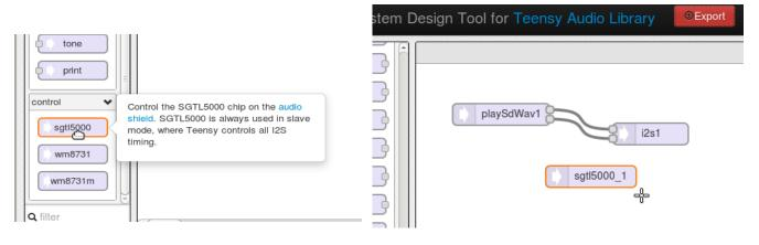
**Step #3:** When you've created an audio system, click the red **Export** button. The design tool will create code which you copy (**Ctrl-C**) from its export window and paste into Arduino.
