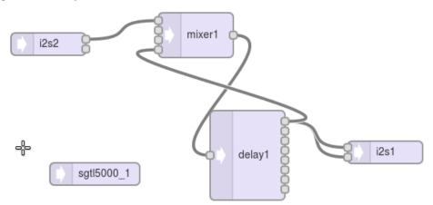
Step #2: When the audio system is designed Export and copy the code to paste in the Arduino sketch
