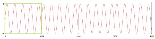
The window function is just another waveform which the signal is multiplied by, before the FFT. The Hanning window is basically just an offset sine wave, which multiplies the original waveform by zero at the beginning and end of the window, and by 1 in the middle.
