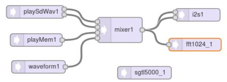
Step #2: When the audio system is designed Export and copy the code to paste in the Arduino sketch
