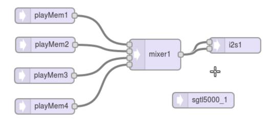
Step #2: When the audio system is designed Export and copy the code to paste in the Arduino sketch
