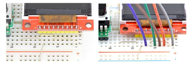
Your breadboard already has the 3 VCC and 1 GND connections installed. Five colored wires are needed to complete the data path.
