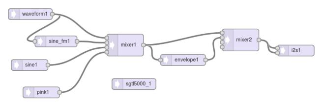
In this system, waveform1 is the "control waveform". It is (usually) a relatively low frequency which controls another signal. Like in the previous example, these mixers are used as switches to allow us to hear one of the 4 synthesized sounds, and to hear it directly or modified by the envelope1 object.
