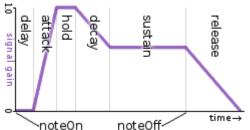
equalizing of pressure between the instrument and musician. The sustain phase is the steady sound heard as the musician continues blowing in the tube. The final release phase emulates the gradual decrease in pressure & sound after the musician stops applying air pressure.
