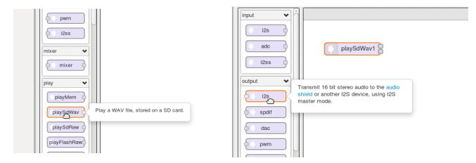
With both objects on the canvas, click (and hold) on their small squares, and drag your mouse to draw wires. Each wire causes a stream of 16 bit, 44.1 kHz audio data to automatically flow between the objects.
