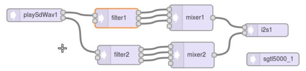
These mixers as a signal routing switch. One channel will be set to 1.0 gain, to pass the signal straight through so we can hear the effect of the filter. The other mixer channels will set to zero to block those signals. The mixers won't actually be doing any "mixing", just routing one of the filter's outputs.
