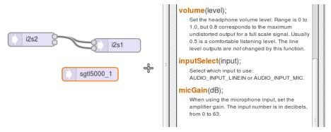
Step #2: When the audio system is designed Export and copy the code to paste in the Arduino sketch
