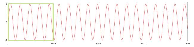
The green box is 1024 points where the FFT analyzes the spectrum. The FFT reports the spectrum based on the assumption the waveform is periodic, that it repeats indefinitely.
