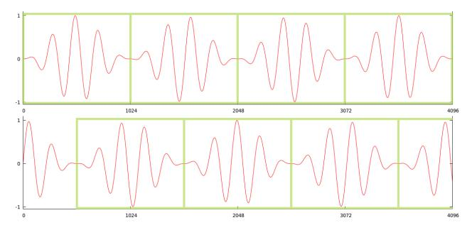
A new 1024 point FFT is completed every 512 samples, because they are performed at twice the rate on 50% overlapping data after windows are applied.
