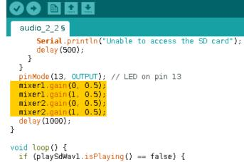
Signals are always be between -1.0 to 1.0. If you mix signals to a sum beyond 1.0, the result is limited or "clipped" to 1.0. Clipping causes harmonic distortion. Gains are usually set to prevent clipping. If you have extra time, try adjusting the gains to experience clipping distortion. Much of the practical experience of audio design is familiarity with the sounds caused by common mistakes.
