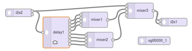
Step #2: When the audio system is designed Export and copy the code to paste in the Arduino sketch
