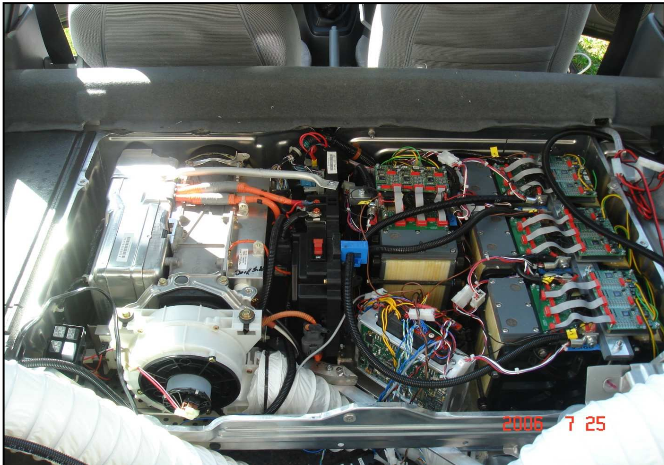
Battery in position (4x36V modules)
