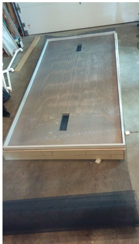
Staple screen to both sides of the absorber frame.
