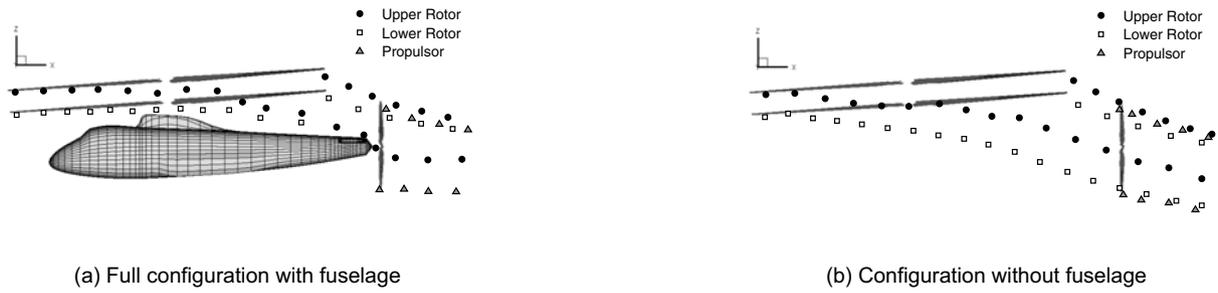
Figure 8. Trajectories of the tip vortices of the main rotors and propulsor at advance ratio  $\mu = 0.15$  showing the points of intersection of individual vortices with the longitudinal plane through the fuselage centreline at various times during a single main rotor revolution.
