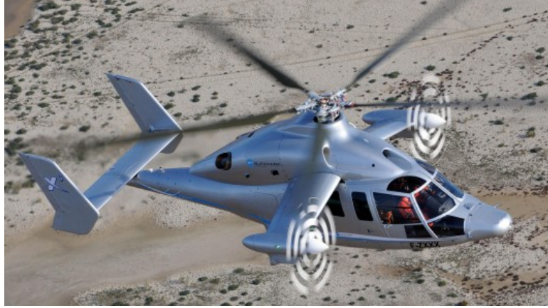
FIGURE 1.1: Eurocopter X3 compound helicopter, which uses a lifting wing with two propellers for auxilliary propulsion [10].
