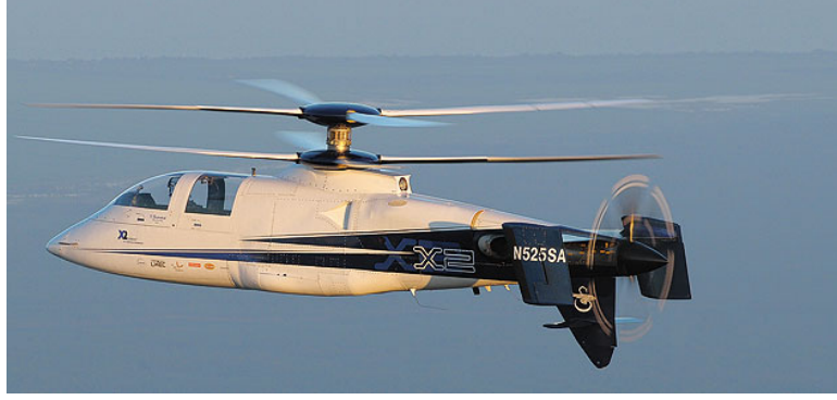
FIGURE 1.2: Sikorsky X2 technology demonstrator, which uses a coaxial rotor and a pusher propeller [15].
